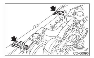
4) Attach power steering hose to the radiator.
