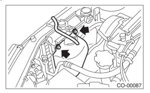
12) Disconnect radiator inlet hose from engine.
