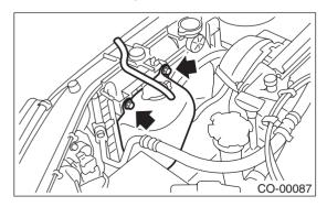
7) Install air intake duct.
