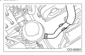
15) While slightly lifting radiator, slide it to left.
