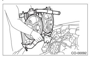
3) Install radiator brackets and tighten bolts.
