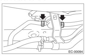
6) Remove pressure control solenoid valve from bracket.
