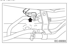
5) Disconnect two evaporation hoses from pressure control solenoid valve.
