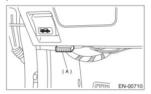
3) Using the general scan tool, call up diagnostic trouble code(s) and freeze frame data.
