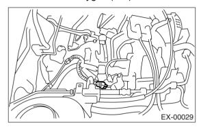
3) Disconnect rear oxygen sensor connector.
