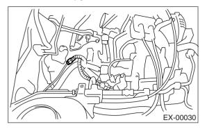
10) Connect front oxygen (A/F) sensor connector.
