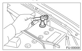
2) Disconnect front oxygen (A/F) sensor connector.
