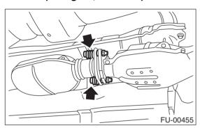
7) Tighten bolt which holds front and center exhaust pipe assembly to hanger bracket.
