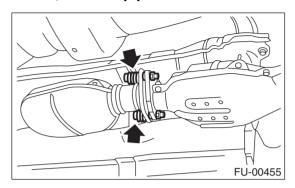
2) Separate rear exhaust pipe from muffler.
