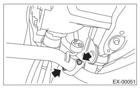
2) Install rear exhaust pipe to center exhaust pipe.
