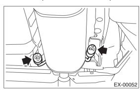
3) Remove front cushion rubber, and detach muffler assembly.
