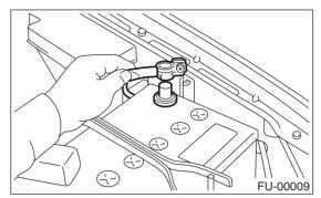
2) Disconnect connectors from engine hanger and front oxygen (A/F) sensor.
