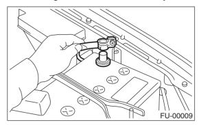
2) Disconnect connector from rear oxygen sensor.
