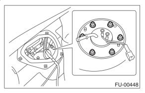
12) Drain fuel from fuel tank by using hand pump.
