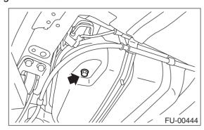
6) Tighten fuel drain plug and install front right side tank cover.
