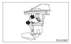
3) Pushing the pawls with a screwdriver, remove fuel level sensor by pulling it downwards.
