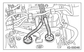
3) Remove spark plugs with the spark plug socket.
