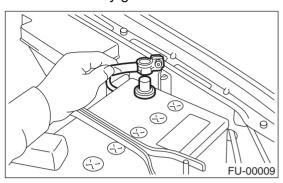
2) Disconnect washer motor connector.
