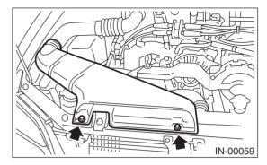
2) Remove bolt which installs air intake duct on body.
