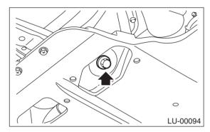
5) Using engine oil of proper quality and viscosity, fill it through the oil filler duct up to upper level on level gauge. Make sure that vehicle is placed level when checking oil level. Use engine oil of proper quality and viscosity, selected in accordance with the table in figure.
