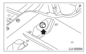
3) Replace drain plug gasket.
