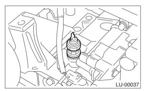
3) Connect terminal of oil pressure switch.
