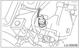
4) Install generator on bracket. <Ref. to SC(H4SO)-15, INSTALLATION, Generator.>
