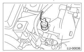
3) Remove oil pressure switch.
