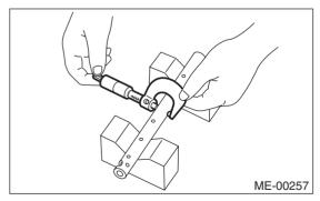
2) If oil clearance exceeds the limit, replace valve rocker arm or shaft, whichever shows greater amount of wear.
