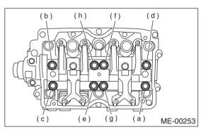
(2) Remove valve rocker assembly.
