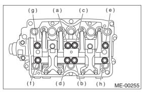
2) Adjust the valve clearances. <Ref. to ME(H4SO)-29, ADJUSTMENT, Valve Clearance.> 3) Install rocker cover and connect PCV hose.
