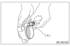
14) Remove coil spring (A) from magnetic switch (B).
