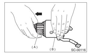
8) Remove screws securing magnetic switch (A) to housing (B).
