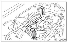
5) Disconnect connector and terminal from starter.
