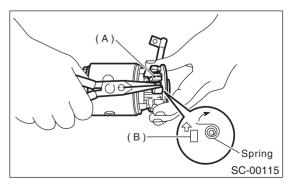
7) Remove armature (A) from yoke (B).
