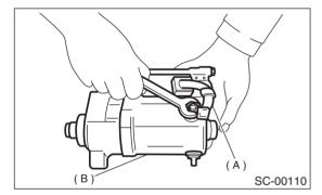
2) Remove through-bolts (A) from end frame (B).
