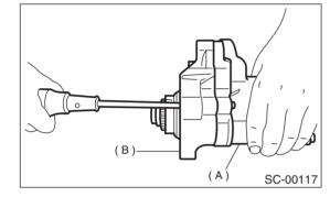
9) Remove housing (A) from magnetic switch (B).
