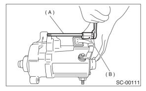
3) Remove yoke (A) from magnetic switch (B).
