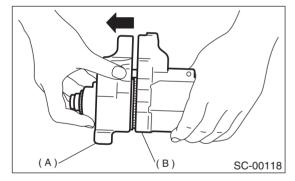
10) Remove clutch (A) from housing (B).
