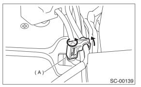
2) Disconnect the positive (+) cable after disconnecting the negative (-) cable of battery.
