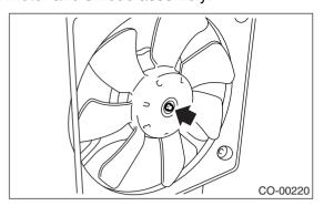
3) Remove the bolts which install the fan motor onto shroud.
