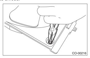
2) Remove the nut which holds the fan itself onto fan motor and shroud assembly.
