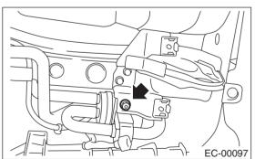
7) Disconnect evaporation hoses, (a) and remove drain filter (b).
