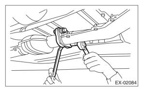
3) Separate the rear exhaust pipe from muffler.
