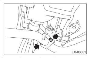
4) Remove the rear exhaust pipe.
