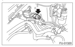
3) Disconnect the engine harness fixed by clip (A).
