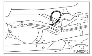
3) Connect the connector to the rear oxygen sensor.
