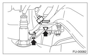
5) Apply SUBARU CRC or its equivalent to the threaded portion of rear oxygen sensor, and leave it for one minute or more.
