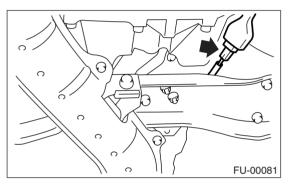
4) Remove the clip by pulling out from the upper side of crossmember.
