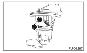
3) Pushing the pawls with a screwdriver, remove fuel level sensor by pulling it downwards.
