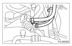
23) Remove the bolts which secure the intake manifold to the cylinder heads.
