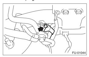
9) Disconnect the evaporation hose and purge valve from the intake manifold.
