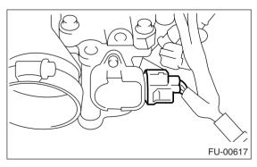
18) Connect the connector to the tumble generator valve actuator.
