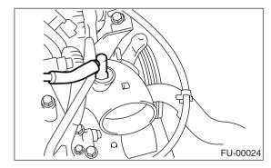
13) Install the power steering pump.
