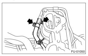
15) Loosen the clamp which holds the right side fuel hose to injector pipe, and then remove the pipe from clamp.
