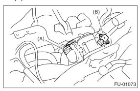
3) Remove the throttle body from the intake manifold.
