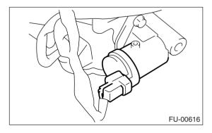
6) Disconnect the connector from the tumble generator valve sensor.
