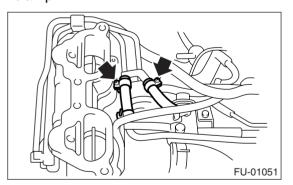
16) Remove the bolts which install the fuel pipe on intake manifold.
