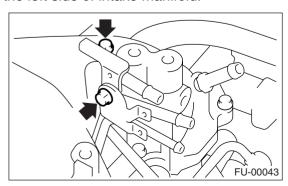
11) Remove the bolt which hold the fuel injector pipe onto intake manifold.
