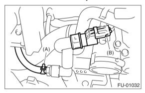
12) Connect the pressure hose to the intake duct.
