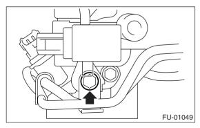
12) Remove the harness bracket which holds the engine harness onto intake manifold.
