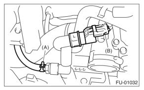
13) Disconnect the engine coolant hoses from the throttle body.
