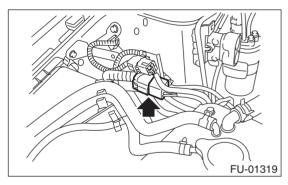
17) Disconnect the connectors from the engine coolant temperature sensor (A), oil pressure switch (B) and crankshaft position sensor (C).
