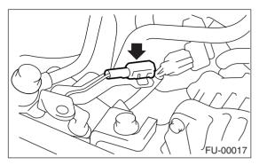
(3) Remove the bolts which secure the power steering pipe brackets to the intake manifold.
