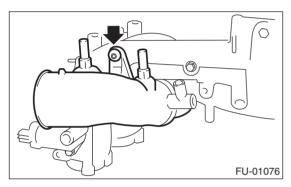
19) Remove the tumble generator valve assembly from the intake manifold.
