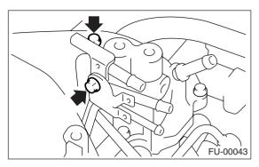
12) Connect the evaporation hoses to the purge valve.
