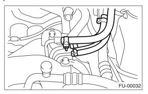
3) Connect the connector to the oil pressure switch (B), crankshaft position sensor (C) and engine coolant temperature sensor (A).
