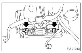
5) Disconnect the connector from the tumble generator valve actuator.
