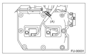
8) Connect the engine harness connector to the bulkhead harness connectors.
