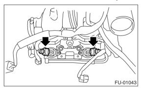
20) Install the throttle body to the intake manifold.
