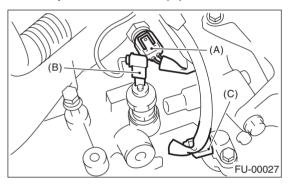
4) Connect the connector to the knock sensor.
