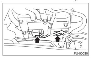
21) Disconnect the engine harness fixed by clip (A) from the bracket.
