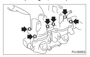
2) Install the air intake duct to the intake manifold.
