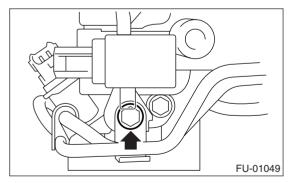
11) Tighten the two bolts which install the fuel pipes on the left side of intake manifold.
