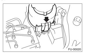
(2) Connect the connector to the power steering pump switch.
