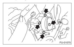
21) Connect the connector to the throttle position sensor (A) and manifold absolute pressure sensor (B).
