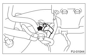
15) Connect the hoses to the purge control solenoid valve.
