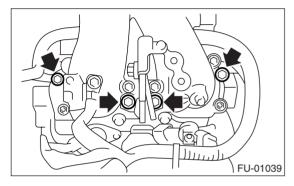
24) Remove the intake manifold.
