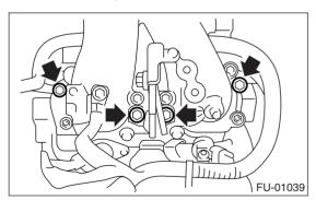
2) Connect the fuel delivery hose, return hose and evaporation hose.
