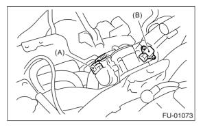
22) Install the engine ground terminal to the intake manifold.
