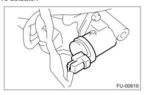
19) Connect the connector to the fuel injector.
