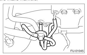
14) Install the purge control solenoid valve.
