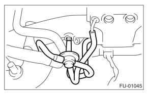
10) Remove the two bolts which hold the fuel pipes on the left side of intake manifold.
