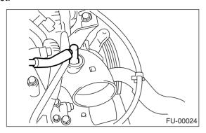
16) Disconnect the engine harness connectors from the bulkhead harness connectors.
