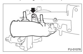
3) Install the fuel pipe assembly and pressure regulator to the intake manifold.
