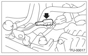
(3) Install the power steering pump, and tighten the bolts.
