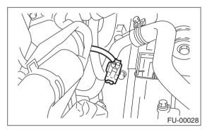
5) Connect the connector to the camshaft position sensor.
