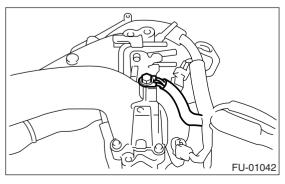
2) Disconnect the connector from the throttle position sensor (A) and manifold absolute pressure sensor (B).
