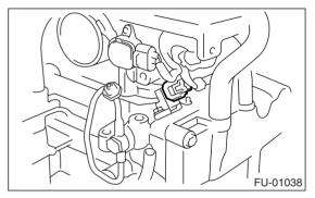
20) Disconnect the connector from the ignition coil.
