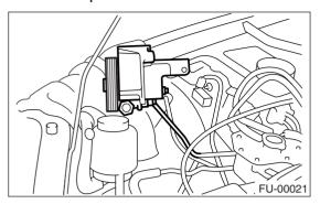
12) Disconnect the emission hose (A) and connector (B) from the PCV hose assembly.
