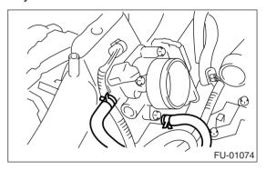
11) Connect the emission hose (A) and connector (B) to the PCV hose assembly.
