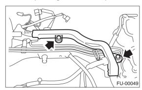
10) Tighten the bolts which install the fuel injector pipe onto intake manifold.
