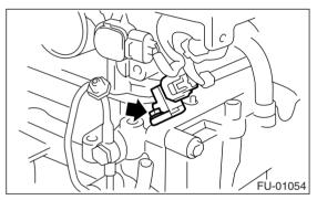
4) Remove the camshaft position sensor LH same as RH side.
