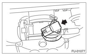
3) Remove the manifold absolute pressure sensor from the throttle body.
