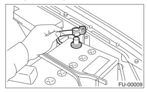
2) Disconnect the washer motor connector.
