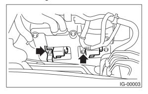
5) Remove the spark plugs with the spark plug sockets.
