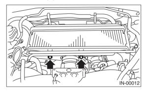
3) Disconnect hose from air bypass valve.
