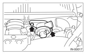
2) Remove intercooler duct from intercooler.
