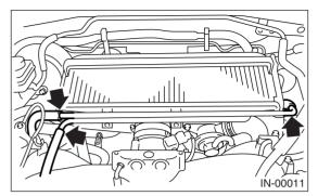
2) Remove PCV pipe from intercooler.
