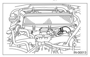
4) Remove bolt which secure intercooler to bracket
