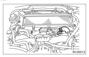
2) Remove air bypass valve from intercooler.
