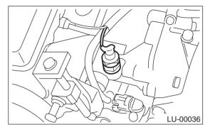
3) Remove the oil pressure switch.
