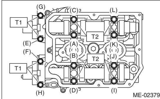
(4) After tightening cap, ensure the camshaft rotates only slightly while holding it at “base” circle.
