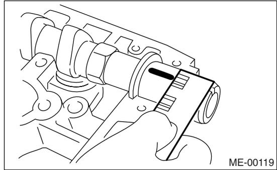
(7) Completely remove the plastigauge.
