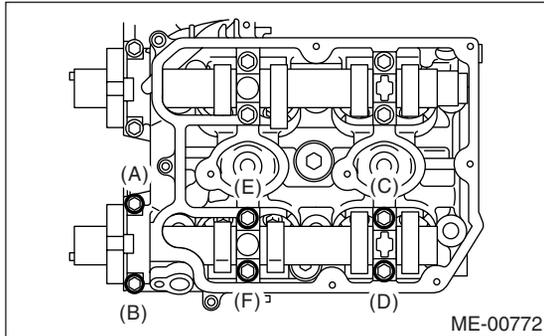
17) Remove the variable valve timing solenoid valve assembly, intake camshaft cap, and camshaft.
