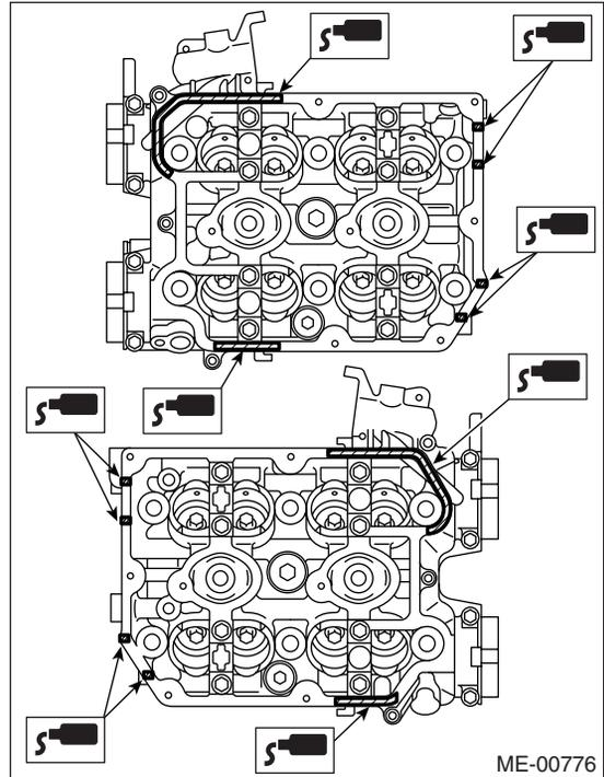
(3) Install the rocker cover on cylinder head. Ensure the gasket is properly positioned during installation.
