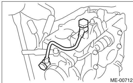
6) Connect the variable valve timing solenoid valve connector.
