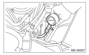
9) Perform at least two measurements per cylinder, and make sure that the values are correct.
