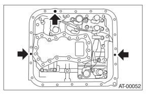
6) Tighten bolts evenly and install the oil pan.
