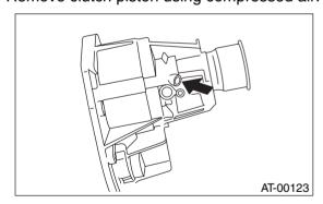
4) Pay attention, not to bend pipe, and remove transfer clutch pipe.
