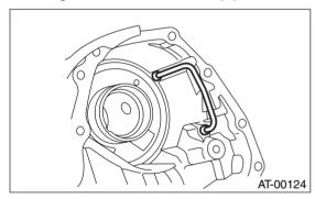
4) Install the test plug.
