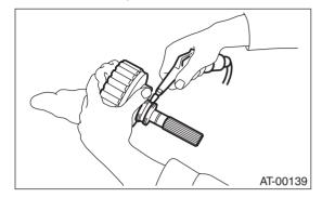
9) Check clearance between snap ring and pressure plate. < Ref. to 4AT-92, INSPECTION.> 10) Press-fit a new ball bearing with ST.
