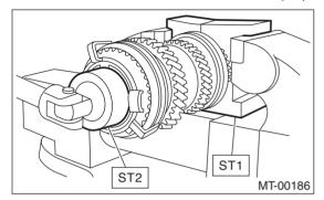
3) Remove the 5th-Rev sleeve and hub assembly, baulk ring, 5th drive gear and needle bearing.
