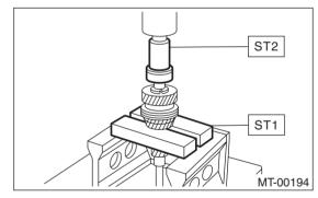
6) Using the ST1 and ST2, install the 5th gear thrust washer and 5th needle bearing race onto the rear section of transmission main shaft.
