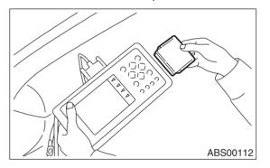
4) Connect Subaru Select Monitor to data link connector.
