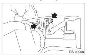
4) Remove bolts which secure link upper to rear arm and detach link upper.
