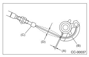
Check that the clearance (A) between throttle cam (B) and lever or cable deflection (D) is within specifications.
