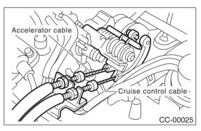
Check movement of the accelerator cable when the cruise control throttle is moved by hand. If NG. check throttle cam.
