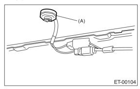
3) Pull the antenna out from roof.
