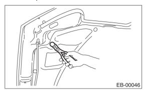
3) Remove bolts to disconnect hood from hinges.
