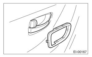
2) Remove two hook (A) of switch panel to remove power window main switch.
