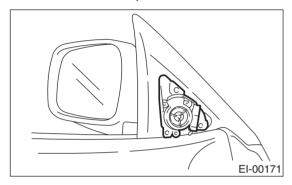
6) Remove seven clips (A) of trim panel using clip remover to remove trim panel.
