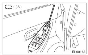
3) Disconnect electrical connectors from power window main switch and mirror switch.
