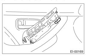
4) Remove three screws and clips.
