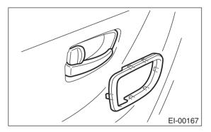
2) Remove two hook (A) of switch panel to remove power window sub switch and disconnect electrical connector.
