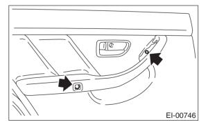
4) Remove seven clips (A) of trim panel using clip remover to remove trim panel.
