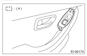
3) Remove two screws and clips.
