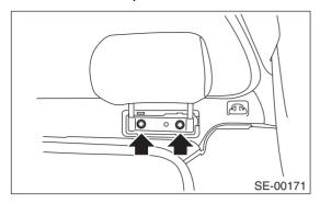
6) Remove cargo net hook and remove rear bulkhead trim.
