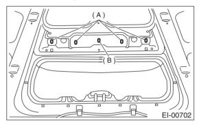
4) Remove eleven clips to remove air duct.
