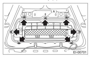
5) Install the hood insulator with new clips.
