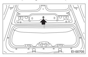
3) Catch three hooks (A) of hood duct to hood holes.
