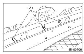
4) Install hood duct with clip (A) and six bolts.
