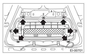
3) Loosen the nut (B), remove four clips (A), and then remove hood grille.
