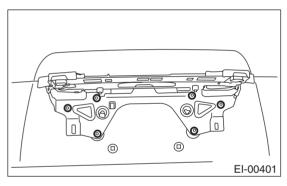
5) Remove clip and bolt and detach tail gate garnish.
