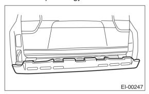
7) Remove bolt and bumper beam.
