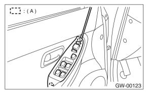
2) Disconnect electrical connectors from power window main switch and mirror switch.
