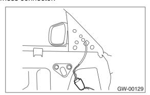
3) Remove screws to remove outer mirror assembly.
