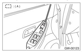
2) Remove four hook (A) to remove remote control mirror switch.
